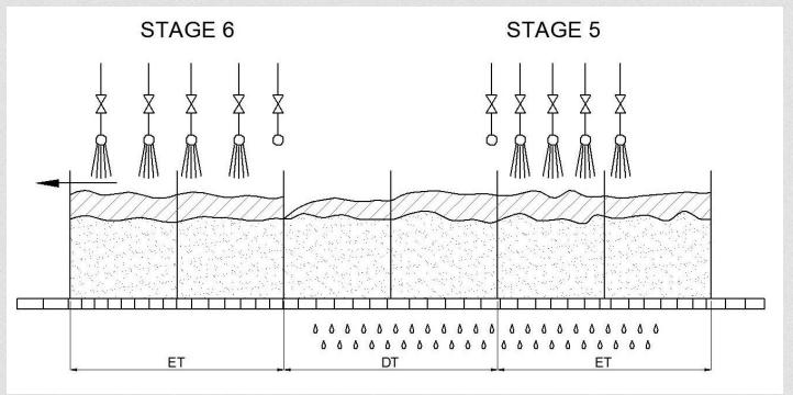
Can change extraction time (ET) and dropping time (DT) when closing some tubes resp. open tubes.
