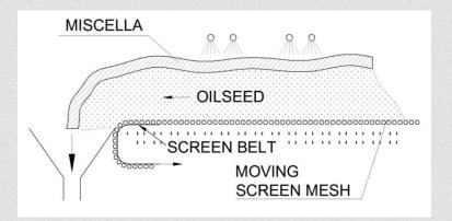
No maintenance of miscella bath; miscella can flow directly to the next stage and to the meal discharge. Less extraction effiency and dangerous of overcarrying to much solvent to the toaster.
