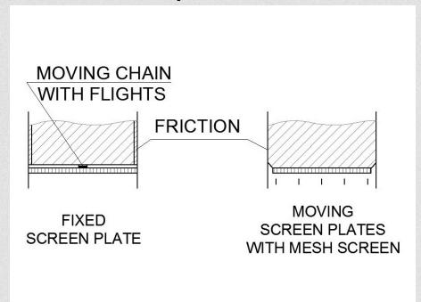
These design give friction between extractor housing and the oilseed. Much wear and tear, which cause shorter life time.
