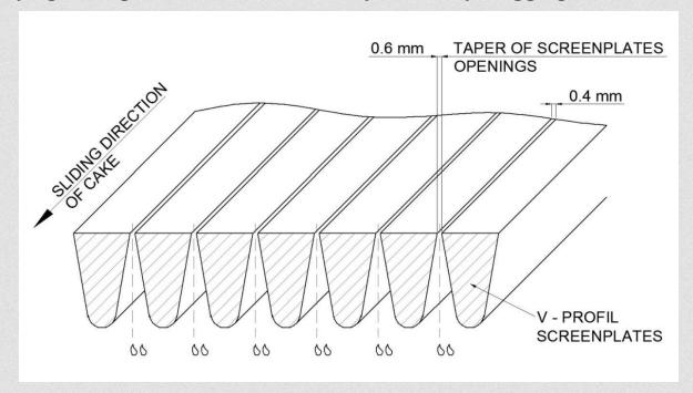
The taper of the screen plate is selected as a function of the oilseed; beeing normally 0,4 – 0,6 mm, to avoid sticking of material at the screen plates.
